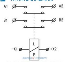
AH Double Pole Double Throw Contactor. (Two Normally Open) A1.A2.B1.B2 Contact Terminal -X1.+X2 Coil Terminal
